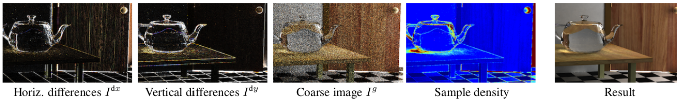
Figure 1: We compute image gradients I^{dx} , I^{dy} and a coarse image I^g using a novel Metropolis algorithm that distributes samples according to path space gradients, resulting in a distribution that mostly follows image edges. The final image is reconstructed using a Poisson solver.
